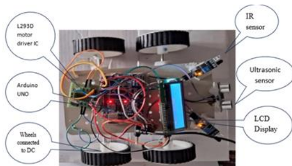
Fig 8: Final Outcome of Autonomous Person Tracking Robot
