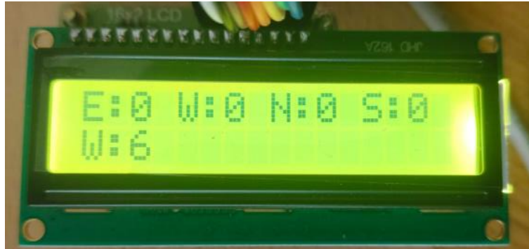
Figure 4: LCD Display Output Showing Real-Time Traffic Status and Signal Information
