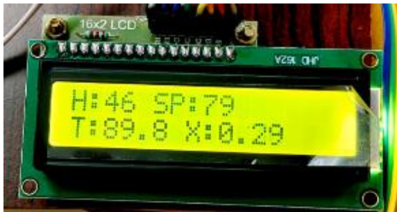
Fig. 4: Heartbeat, spo2, tempreature, mems values displaying on LCD
