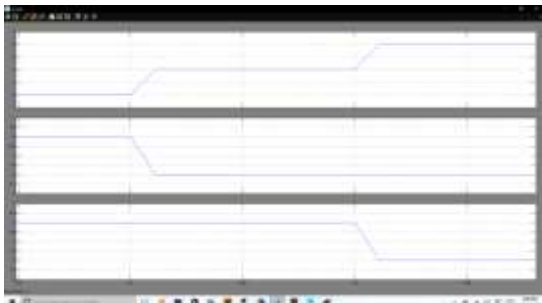
Fig:6- Simulation result of power flow using three seven-level converters ( f_{PWM} = 500 kHz).
