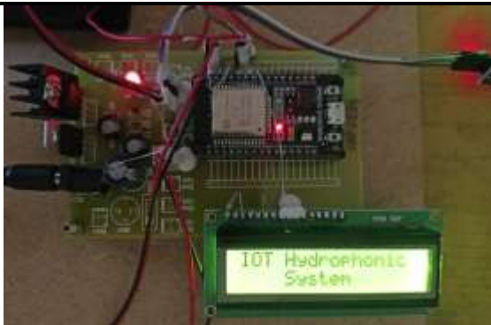
Figure 4. LCD Display Showing IoT Hydroponic System Initialization.
