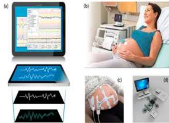
Fig. 1. Fetal healthcare monitoring. (a) a digital monitoring interface, (b) a pregnant woman using a wireless clinical setting, (c) an abdominal patch with integrated electrodes, and (d) components of a portable fetal monitoring kit.
