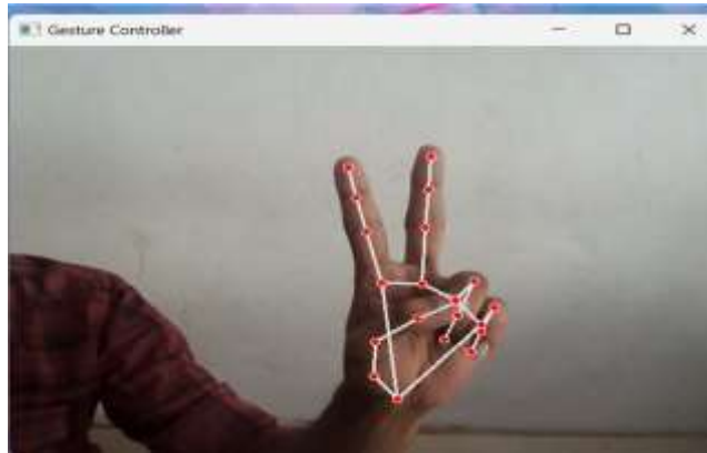
Fig.5: hand gesture detected as cursor movement.
