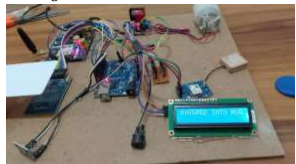
Fig.6.2: Bus Ticketing Prototype Displaying 'Entered Into Bus' Status
