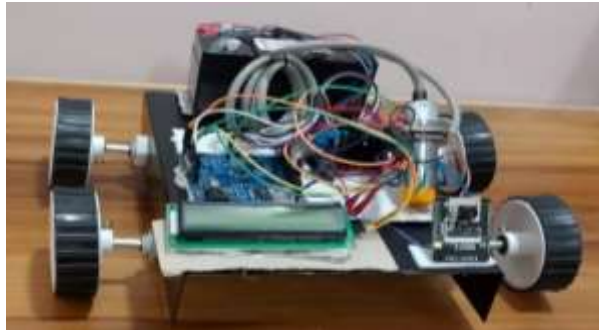
Fig. 6.1: Bomb Disposal Robot Prototype Chassis
