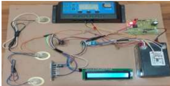
Fig. 6.1: Piezoelectric Hybrid Charging Hardware Prototype
