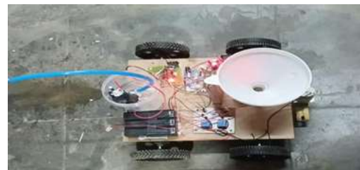
Fig 10: Module for seed dispenser machine
