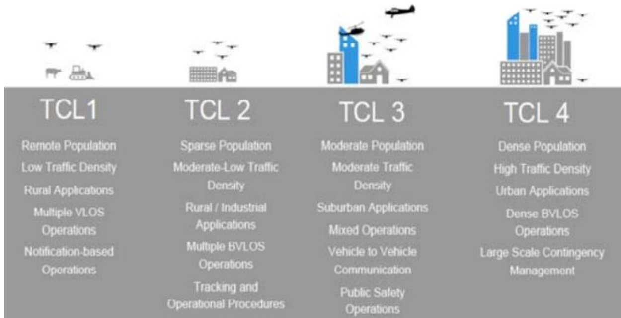
Figure 4 The four-stage planning and phased goals of the UTM UAV Technical Capability Level (TCL)[612]
