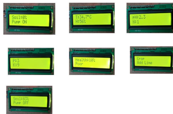
Fig. 7. LCD outputs for measured conditions, pump state, crop advisory, and soil-health information.
