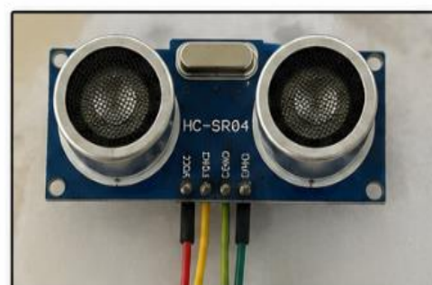
Fig. 6.4: Ultrasonic Sensor for Distance Detection
