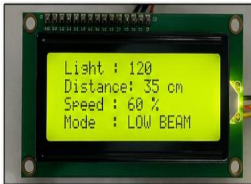
Fig. 6.7: LCD Display Showing System Output
