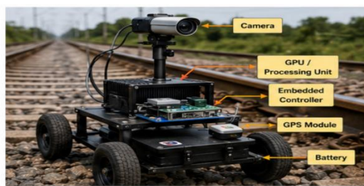
Fig. 6.1: Railway Track Inspection Trolley Hardware Setup
