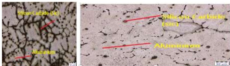
Figure 9: Al & SiC, Micro-structure at 800°C
