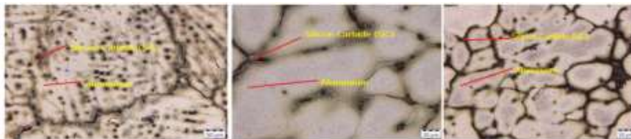
Figure 11: Al & SiC, Micro-structure at 1200°C
