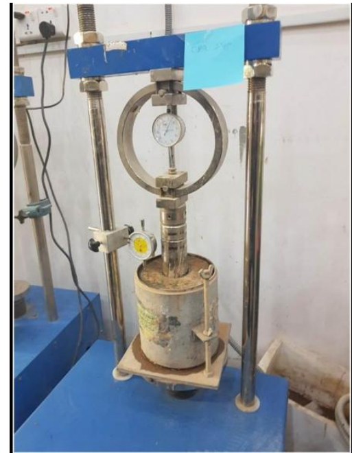
Figure 4. California Bearing Ratio (CBR) Test
