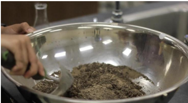
Figure 3. Preparation of Stabilized Soil Mixture
