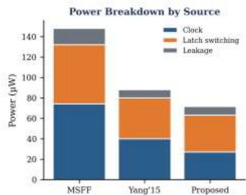
Fig. 11. Power decomposition by source at 500 MHz.
