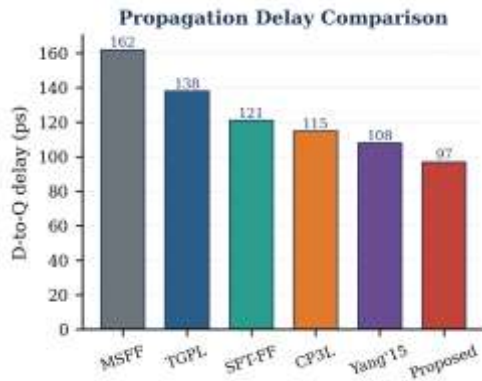
Fig. 7. Data-to-Q propagation-delay comparison.
