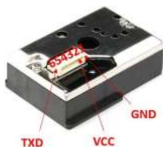
Fig. 6. Fine particulate matter sensor module (GP2Y1010AU0F). SHARP created the sensor used to measure the fine particulate matter (PM 2.5 ) concentration in this investigation, namely, the GP2Y1010AU0F model
