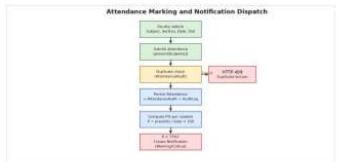
Fig. 3. Attendance marking and notification dispatch workflow: Faculty submits → Duplicate check → Persist Attendance + Audit → Compute P per student → Dispatch Notification → Faculty receives confirmation
