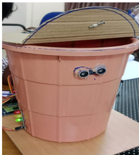
Figure 3: Automatic Lid Operation and Ultrasonic-Based Smart Waste Bin Prototype
