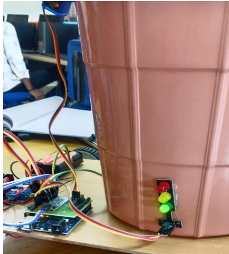
Figure 4: Status Indication and Embedded Control Unit of the IoT Smart Waste Bin
