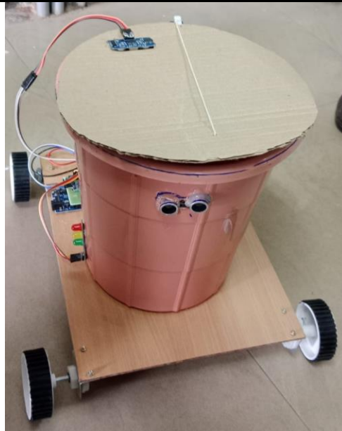
Figure 2: Prototype Implementation of the IoT-Based Smart Waste Bin System
