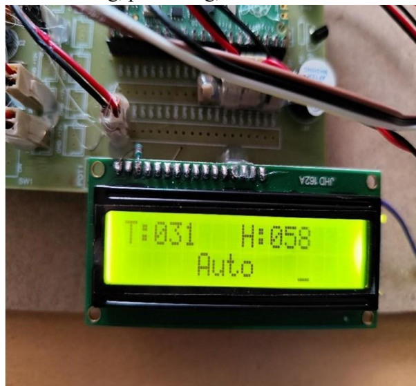
Fig. 5. LCD Display Showing Real-Time Temperature, Humidity, and Auto Mode Status
