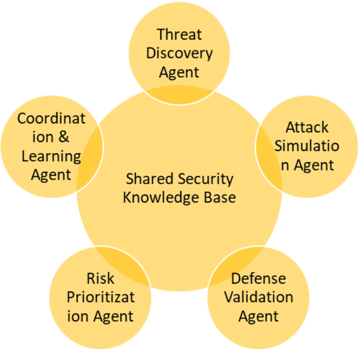
Figure 9.3: Multi-Agent Security Testing Architecture
