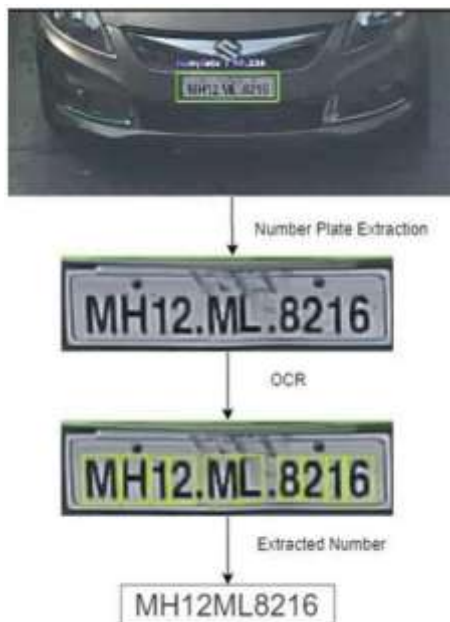
Figure 9: shows the detection of the number plate of the vehicle, then the characters are read using OCR
